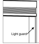
b. When light guard exceeds certain length, it will be spliced into 2 pieces. We recommend that the seam be placed as close to the fabric stack as possible, as shown in below drawings.
